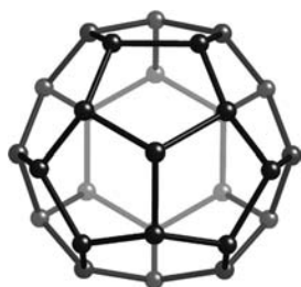
Figure 1. The structure originally proposed for a C_{28} fullerene. It contains four units of directly triple-fused pentagons arranged in tetrahedral symmetry.
